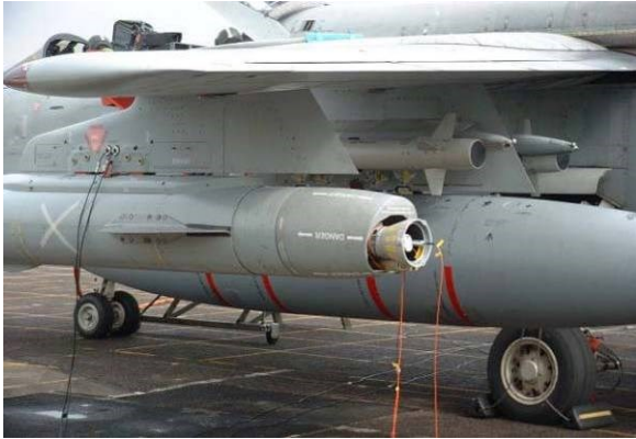
EED testing on a Tornado aircraft
